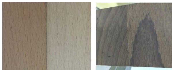
Figure 2. Steamed (left) and heat treated (right) beech wood
