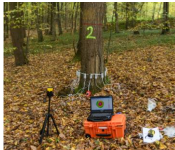
Figure 1. Acoustic tomograph ARBOTOM
