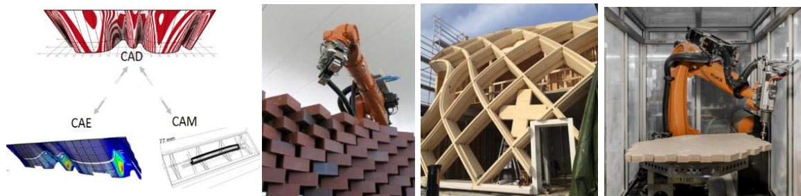
Figure 1. Developing the geometry, designing the supporting framework, and generating production data are all decentralized yet interconnected processes. An integrated data exchange with clearly defined interfaces makes seamless project management possible.
