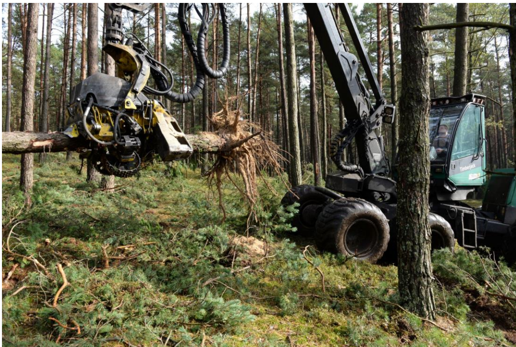
Figure 1. The machine-assisted combined roundwood harvesting, including stumpwood. Source: Own elaboration based on [author's photos by Wladyslaw Kusiak, Notecka Forests]
