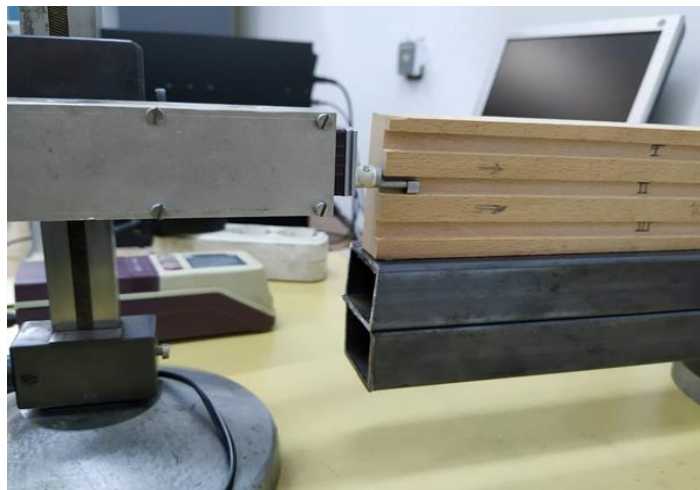
Figure 6. Measurement of surface roughness
