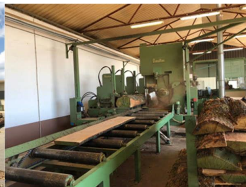
Figure 2. Log band saw used for sawing
