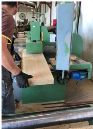
Figure 3. Circular saw with laser for longitudinal sawing.
