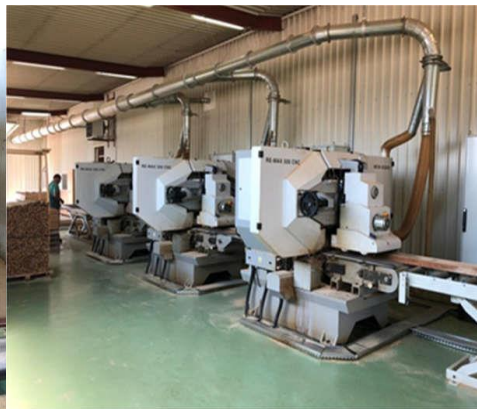
Figure 4. Line of multiple horizontal narrow-blade band saws
