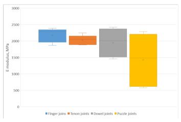
Figure 6. Distribution of E modulus results of end-to end grain joints
