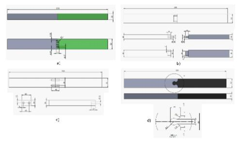
Figure 1. End-to end grain joints: a) finger joint, b) tenon joint, c) dowel joint, d) puzzle joint
