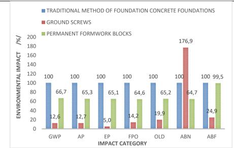
Figure 23: Environmental impact for selected bases in percentage. Abbreviations used: GWP (Global warming potential), AP (Acidification potential of soil and water), EP (Eutrophication potential (Eutrophication)), FPO (Formation of Photochemical ozone), OLD (Formation of Photochemical ozone), ABN (Abiotic depletion potential for non-fossil resources), ABF (Abiotic depletion potential for fossil resources).
