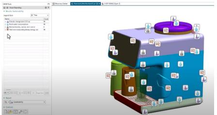
Figure 2. Visualisation of the environmental impact for each component of the assembly in NX Sustainability impact assessment
