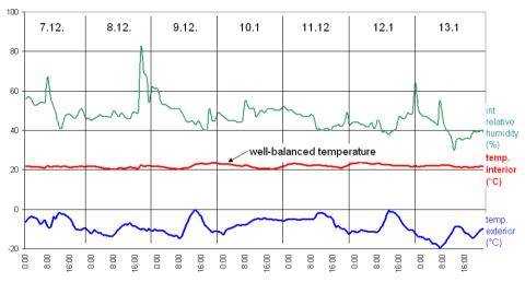
Figure 5. A winter week - internal and external temperatures, bathroom
