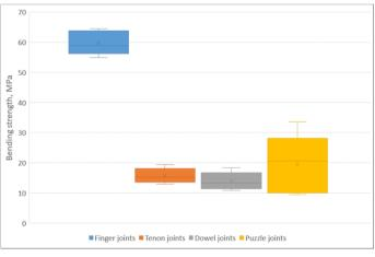
Figure 4. Distribution of bending strength results of end-to end grain joints
