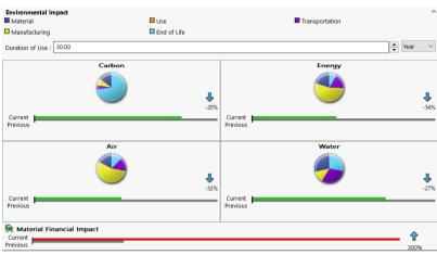
Figure 1. Graphical visualisation of LCA results in Solidworks Sustainability
