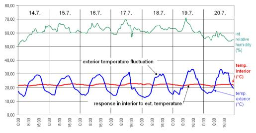
Figure 7. Hot summer week – internal and external temperatures, room
